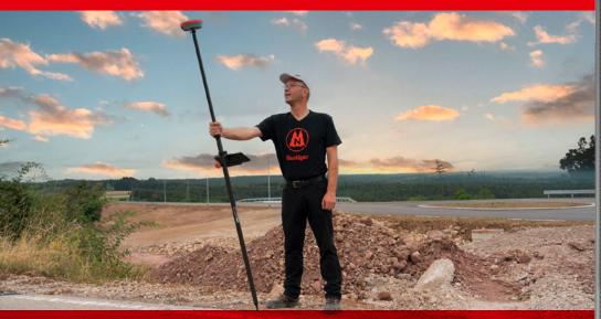
GNPS-42 System for real-time positioning (RTK) for recording and staking out points and geometric shapes for
